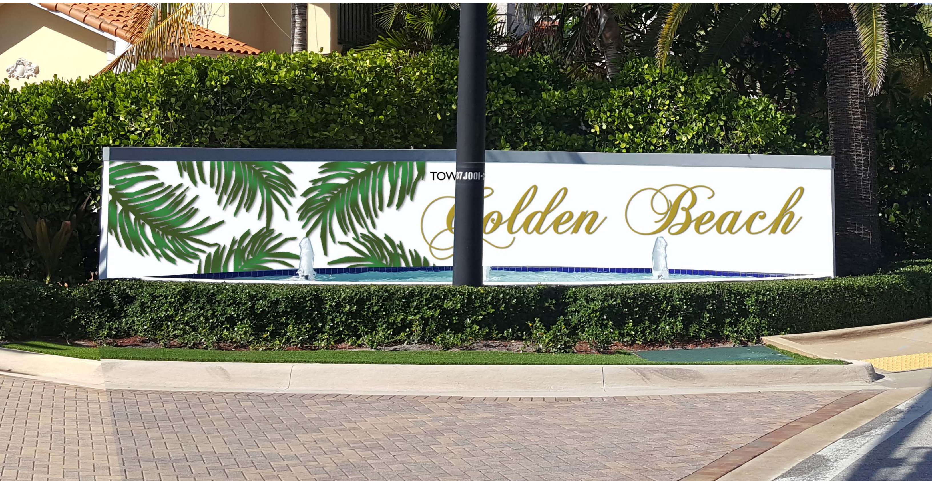
Concept 2: Laser Cut Metal Letters on White Stucco Wall with Laser Cut and Bent Metal Palm Fronds Painted Green
