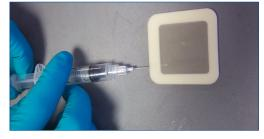
Thorough inspection for salt contamination (including chloride concentration measurement) ensures optimum surface preparation
