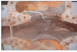
Corroded and cavitated pump
