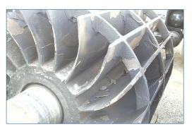
Damaged rotor before rebuilding
