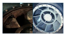
Diffuser vanes with steel gauze in place
