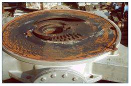
Erosion-corrosion damage on port plate
