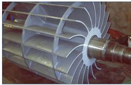
Application of Belzona 1311 and Belzona 1321
