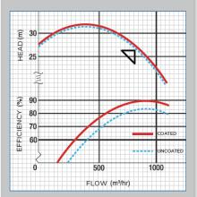
For this test, a single stage, end suction centrifugal pump with 10 inch suction and discharge branches was chosen. In uncoated condition and running at 1300 rpm, the pump was found to deliver 875m<sup>3</sup>/hr at 26.5 meter head with an overall peak efficiency of 83.5%.
