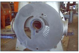
Port plate repaired with Belzona 1111
